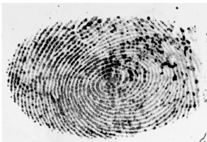
Fingerprint treated with polycyano (365 nm excitation, 400 nm UV cut filter).
